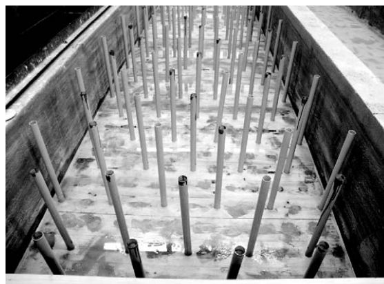
Fig. 1. Laboratory flume with 12.8 stems of artificial vegetation \text{m}^{-2} .
